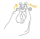
**16.** On the external bench side, fit the Electronic Board into the clips of the plastic cover.
