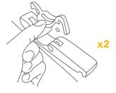
**03.** Remove dirty or worn out Power pad from the Paper Bar Support.
