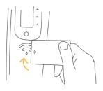
**03.** Pass again the card to validate the installation, until you hear the acoustic signal.
