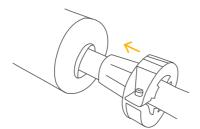
**42.** Introduce the cone into the paper roll.
