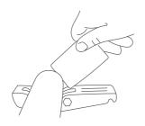
**52.** Check the contact between the bar and the Cap with the help of a card or a thin cardboard (the card should not slide between the two parts).
