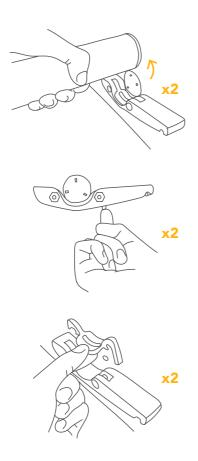
**01.** Remove the Paper Bar from lateral feet of the plotter.
