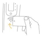
01. Get the option card and pass it through the RFID zone (on the right side panel) for at least 2 seconds, until you hear the acoustic signal.
