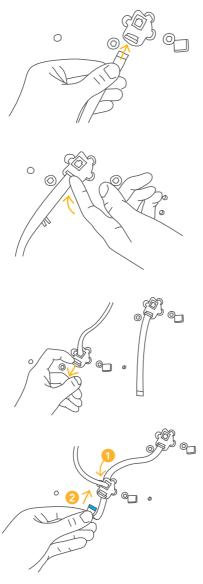
18. Connect the Flat Cable into the connector.Take care of the cable position!
