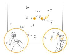
**13.** Fasten the Support. Hold the nuts with your fingers to fix it well.
